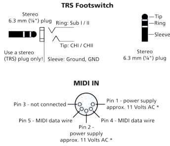
\*: AC voltage is routed to Pin 1 and Pin 2 only when the Phantom Power switch is engaged.
