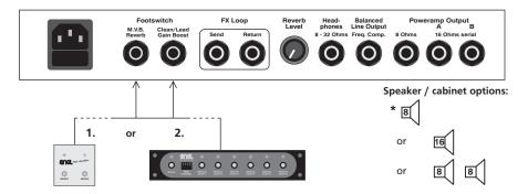
Use a dual footswitch such as the ENGL Z-4, connecting it to the amp via a stereo cord equipped with ¼" jack plugs. You can switch channels and *Gain Boost* via the dual footswitch connected to port 17, *M.V.B.* and *Reverb Off/On* via the dual footswitch connected to port 16.
